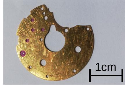
Fig. 1. Watch component used for pick up and assembly in the COB’HOOK project.
